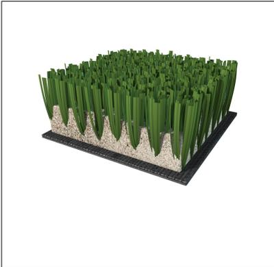
Latest generation artificial turf, manufactured with the TUFTING system. It has a gauge of 3/16" with 26 tufts/dm, resulting in 54.600 tufts/m<sup>2</sup>. The STx available in different colors turf filament has a height of 12 mm and 9.000 Dtex.
