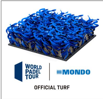
Latest generation artificial turf, manufactured with the TUFTING system. It has a gauge of 3/16" with 22 tufts/dm, resulting in 46.200 tufts/m<sup>2</sup>. The Supercourt XN available in different colors turf filament has a height of 10 mm and 10.000 dtex.
