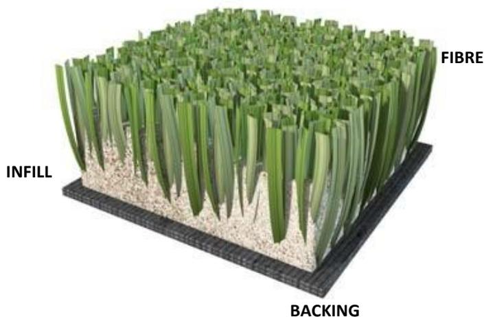
The structure of the artificial turf surface has three basic elements:
